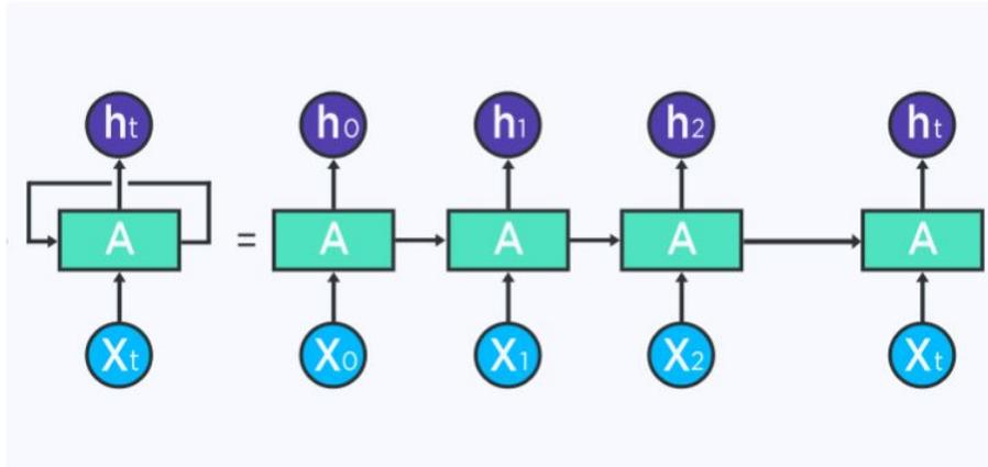
RNN is unrolled after the equal sign. Note there is no cycle after the equal sign since the different time steps are visualized and information is passed from one time step to the next. This illustration also shows why a RNN can be seen as a sequence of neural networks. Within BPTT the error is backpropagated from the last to the first timestep, while unrolling all the timesteps. This allows calculating the error for each timestep, which allows updating the weights.
