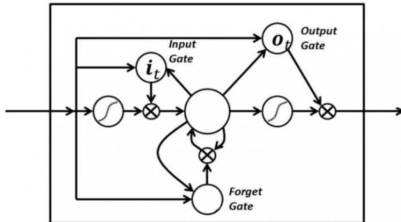
are analog in the form of sigmoids, meaning they range from zero to one. The fact that they are analog enables them to do back propagation.
